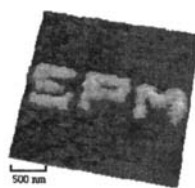
Fig.2 Piezoresponse image of “SPM” pattern domain formed by vector scanning the probe tip.
